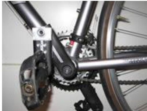
Figure 7: Pivoting Crank Arm
